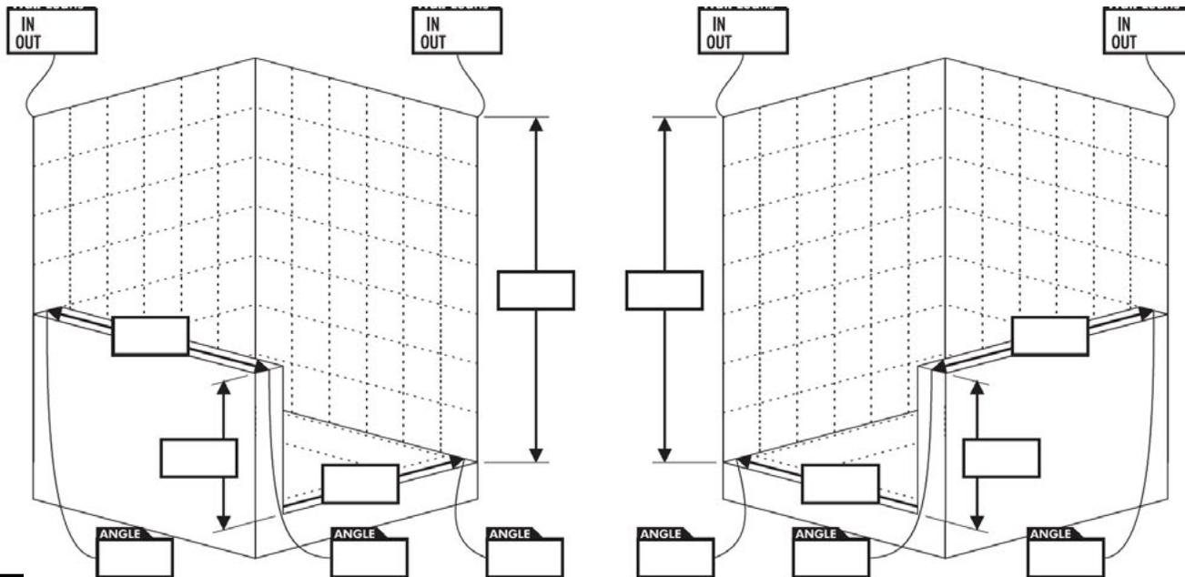
**NOTE:** This layout is for an enclosure with a return on a buttress, with **NO NOTCHED PANEL**. For a notched panel that joins a return, refer to page CMS.04E.
